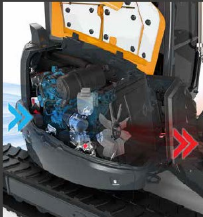
REVERSIBLE FAN KEEPS YOUR MINI PROTECTED A standard feature that prevents dust buildup on the radiators and ensures more efficient cooling of the machine's main components.
